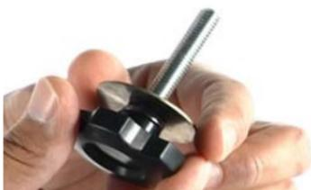
**STEP 8:** To assemble the Adjustment Bolt, hold the parts in your hand in this order: Small Washer; Ball Bearing; Large Washer. Place them on the threaded bolt in that order, with the small washer closest to the plastic knob.
