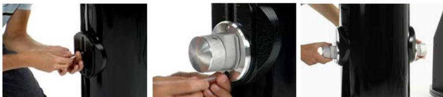
**STEP 1:** Remove the (2) bolts found on the opening on one side of the OTA. This is where you will connect the silver Side Bearing. Align the bearing (top bolt first) and tighten into place. Repeat on the other side of the OTA.
