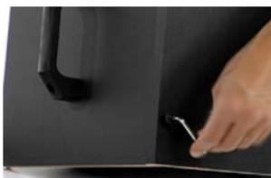
**STEP 2:** Connect the Base Front to the Left Base Side using the pre-drilled holes in the Base Front and (2) Long Black Allen Screws
