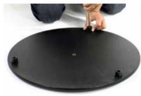
**STEP 5:** First, the feet must be attached to the Base Plate. Choose the Base Plate with (1) center hole and (3) holes around the edge. **IMPORTANT:** The feet must be attached to the side with a brass center hole. Screw all (3) feet in place, with the wider side facing the board, using (3) medium silver Phillips screws.
