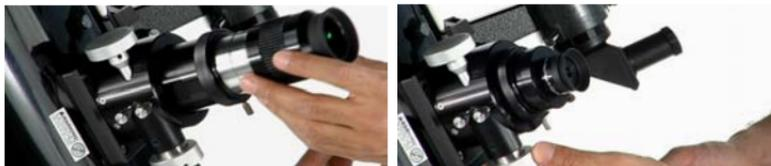
1. The 2-inch eyepiece format is the largest. 2 inches is the diameter of the eyepiece tube, measured on the chrome side.
