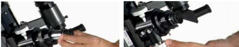
1. The 1.25-inch is the most commonly used eyepiece format. The measurement of 1.25 inches is the diameter of the eyepiece tube, measured on the chrome side.
