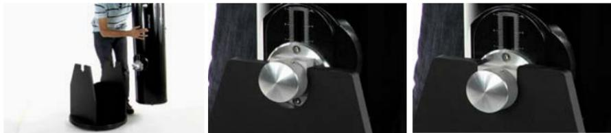
**STEP 2:** You are now ready to place the OTA onto the Base Assembly. Be sure to have the base assembly ready to align with the OTA before you lift the optical tube. The indentations on the Base Assembly will perfectly fit the silver Side Bearings on the OTA.
